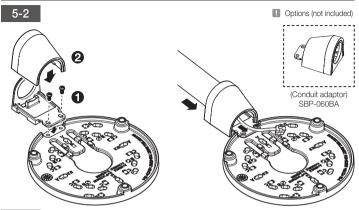
Installing network cable (XNO-A9084R/XNO-A8084R: IP66/IP67)
