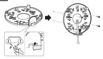
5-1 • Installing using pipe
